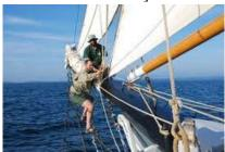
Not all boats have a bow pulpit. It is not practical for most catamaran designs and also on boats with a long *bowsprit* [a pole or platform that extends well ahead of the boat's bow from which jibs and other headsails are flown.] In these cases special netting may extend along
